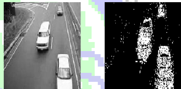
Fig.2. Detection of moving objects using GMM method
