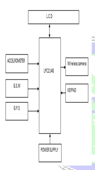
CASE1: If the accelerometer angle is in between a1 and a2 "FIRST" message should be forwarded to stored 3 mobile numbers along with its location.
