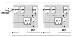
The above block diagram shows the power controlled Ring counter. First, total block is devided into two blocks. Each block is having one SR FLIPFLOP controller
