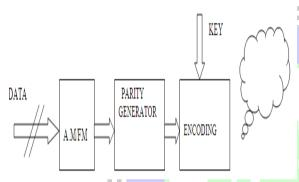
In order to send data in space, data is needed to be modulated. For that purpose, we are using Amplitude modulation. Error detecting codes should be added to detect any error occurred in space or not. Here, even parity generators are used for that purpose. After that encoding should be takes place to prevent data from hackers. One separate key is used for that encoding purpose. Yielded data is XOR'ed with key to get encoded data.
