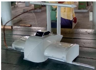
Figure 6: WIG craft model with endplates
