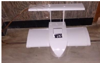
Figure 4: New compound wing configuration.
